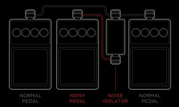
Place the Isolator between the power supply output and the input of the noisy pedal using the included power patch cord. MAXIMUM POWER DRAW IS 500MA. DO NOT EXCEED.
