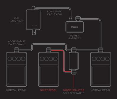
Certain combinations of pedals can cause noise issues especially when mixing analog and digital pedals. The Pedal Noise Isolator (PW-XPNDPNI-01, sold separately), can silence a noisy pedal by providing true galyanic isolation.
